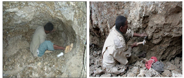
Figure 3. Miners at Wegel Tena use crude materials as hammer and chisel shown here, to extract opal from the exposed seam along the canyon's flank.
