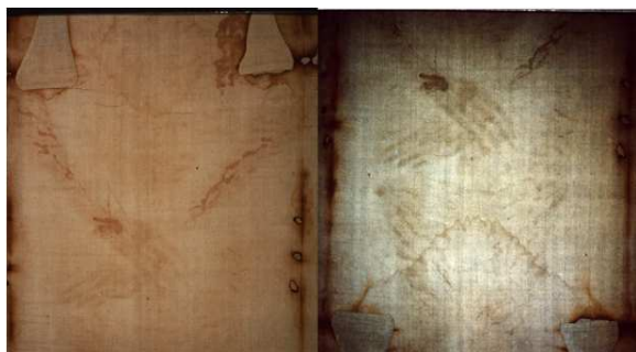
Figure 6. Hands and upper legs area. Left: white light, right: UVF. Hands and body areas are absorbing (rather than fluorescing) as is the triangular water-front. Faint scorches covered by the patches fluoresce reddish.
