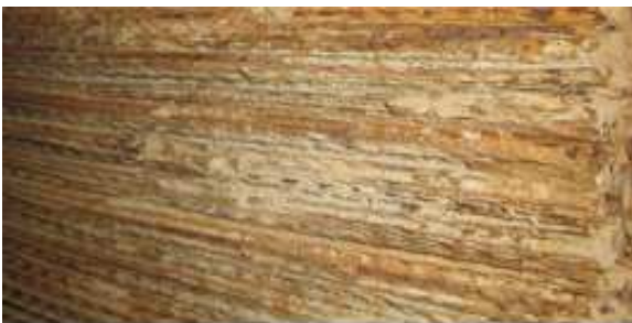
Figure 2. Plugging condition at the lower part of regenerator in the Middle Temperature section.
