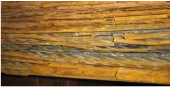
Figure 1. Wear condition of regenerator in the High Temperature section of air preheater.
