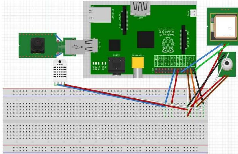
Figure 1. Circuit-aided design (CAD) of connection of components.
